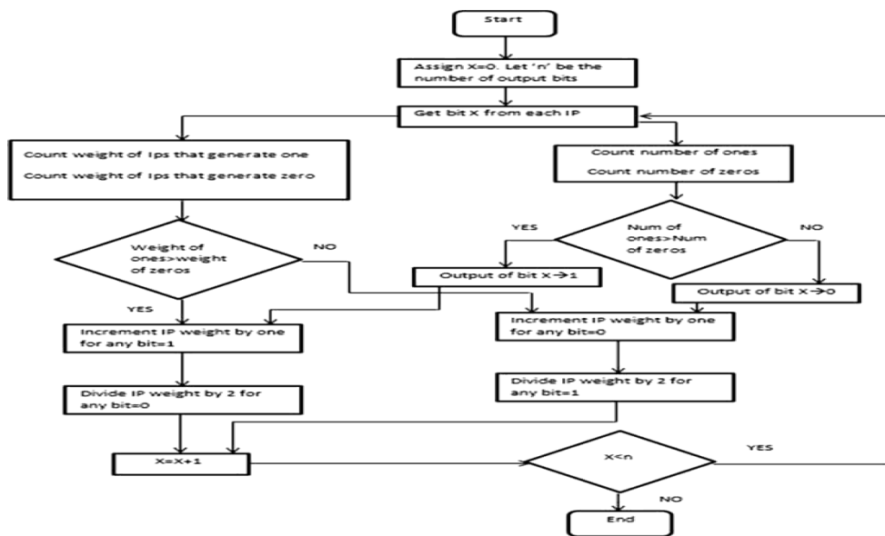
Fig 5.1 Flowchart of modified-weighted voting algorithm
